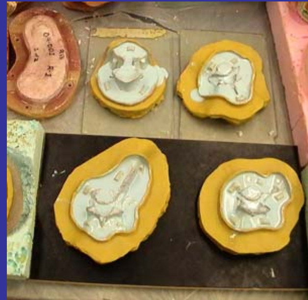
Original bones set in clay, laminated with silicone rubber, and mother molded with polyester + fiberglass
