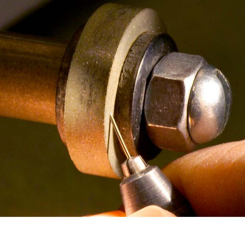
The needles are sharpened on this diamond impregnated rubber wheel that is mounted on a miniature Foredom bench grinder. The wheel rotates away from the acute edge and final touch-up is done on silicone carbide wet or dry sandpaper 1000 grit or higher.
