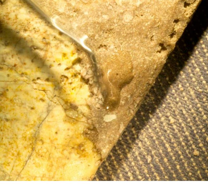
(11) The pick slides along in contact with the work so the maximum amount of fluid will transfer from it.
