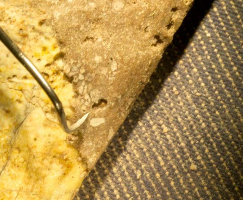
(7) Everything must be done in a quick but fluid motion under the 'scope. This is a dry run to visually locate everything so there will be no searching to bring the pick into the field of view during the real thing. The object, in this instance ,is to fill the void seen at the sharp end of the pick. But the same method is used in filling cracks. The specimen rests on a sandbag made of denim.
