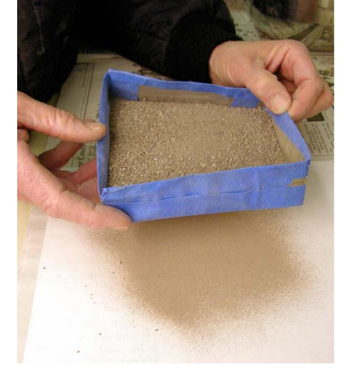
(5) Some of the large grain fraction is then put through a 30-mesh strainer producing the fine grain fraction. What we are producing is something like the sand and gravel used as aggregate to mix with portland cement and water to make concrete. They make it stronger. Another similarity here is that by using only the fine grain fraction a sort of superglue mortar is produced for filling and adhesion in very small gaps.
