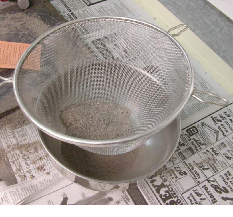
(4) The rubble is then put through a 14-mesh (14 openings to the inch) kitchen strainer.. This produces the large grain fraction of the aggregate we will use. It is what you see in the bowl under the strainer.
