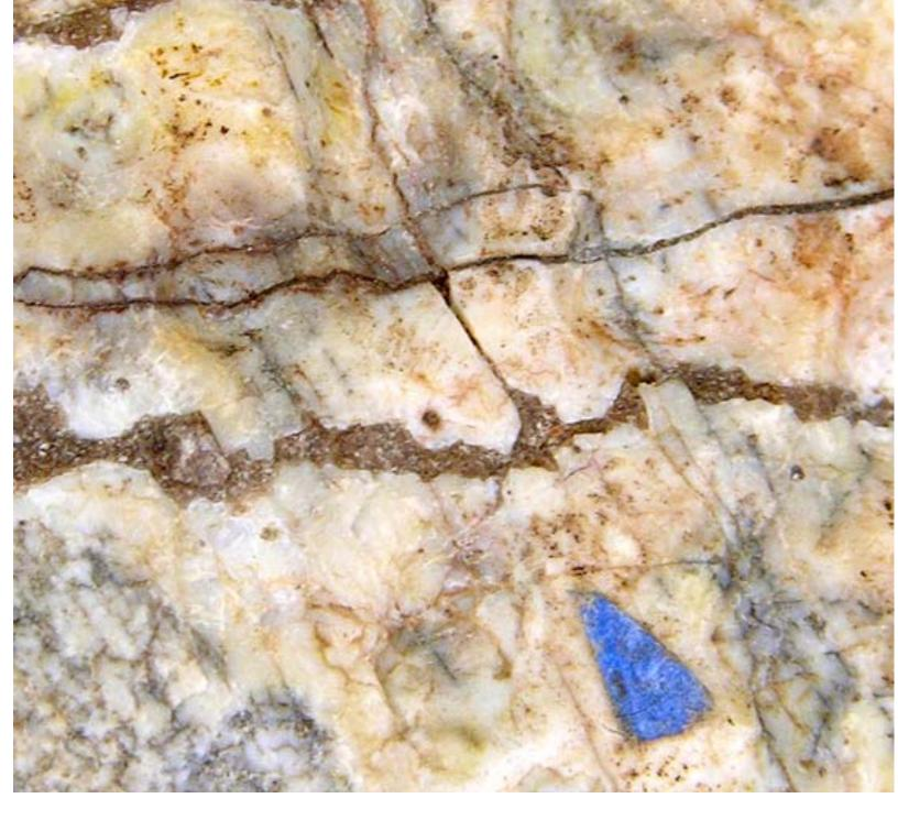
The same shot after the filler has been carved to surface contour. The amber patches at the top of the image are old consolidant that will be removed the same way.
