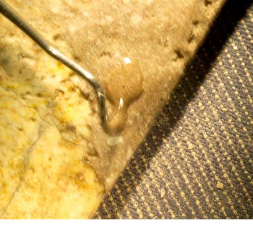
(10) Contact is made and in the same motion the pick is moved towards the void so, in the second or two remaining, the fluid will fill it from the bottom up as it flows in, and avoid trapping air.
