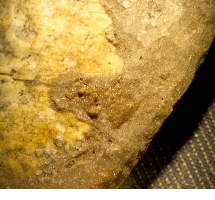
(15) The resin has fired and the mixture now fills the hole and has shrunk in volume.
