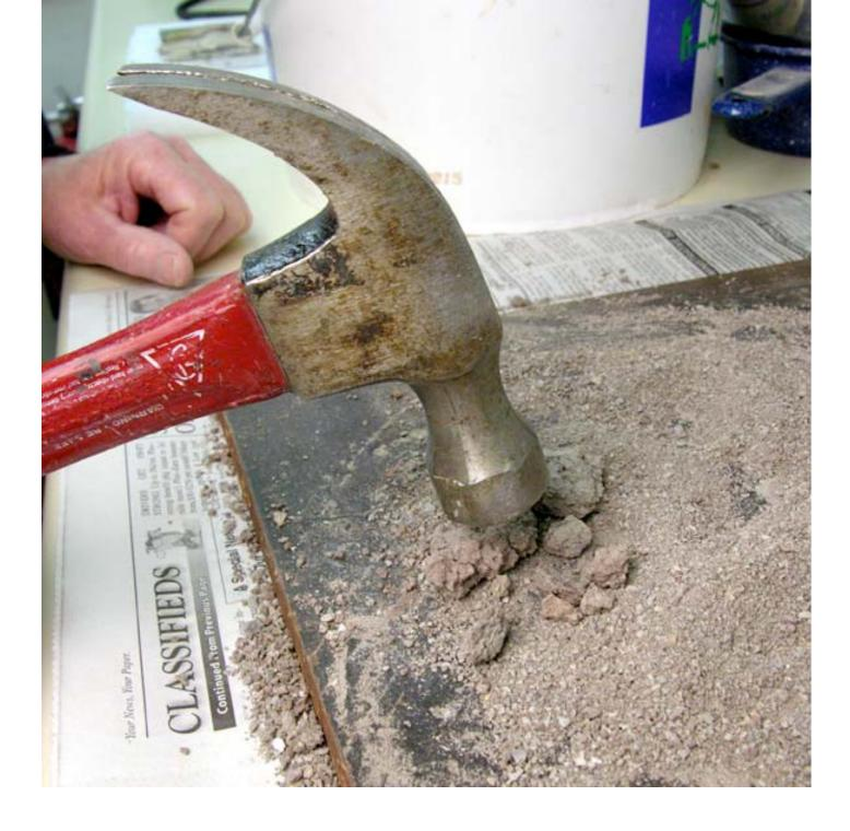
(3) Matrix, processed to make aggregate for the system, was pounded with a hammer on a steel plate and the crushed rubble swept onto the newspaper underneath it.
