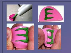
Finally we used a product called Vinyl Polysiloxane to write on an existing mold using a dental syringe. Although the Polysiloxane did not spread like the silicone, it was not possible to write in a small font size. The compound did stay intact and stuck to the silicone after repeated attempts to remove it.
