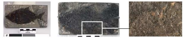
Images of the untreated sample on the left and the sample coated with an uneven layer of molten CDD on the right seen as the darker surface areas. Too much CDD was delivered to the bottom of the sample while the top was not fully coated. The detail shows areas of crystal formation making it unsuitable for molding.
