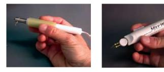
Kistka electric stylus (left) was found to be useful for delivery of minute amounts of CDD. The Super Max Wax Pen (right) was good for re-heating areas coated with CDD to improve flow.
