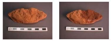
We were unable to successfully consolidate porous sandstone matrix using CDD. The uncoated sample is seen on the left and the partially coated sample on the right.
