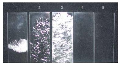
Testing for residues by application to glass slides
