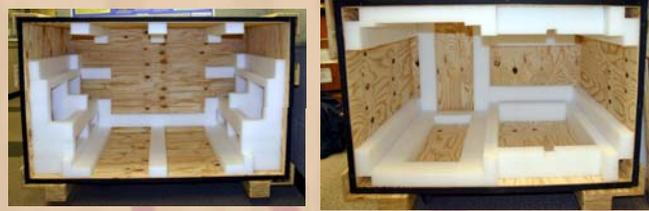
Figure 3: (above) The two crates fabricated by Icon Group, Inc. Internal view shows lid gasket and ethafoam padding used to secure the foam boxes. (below) Foamcore boxes secured within the crates.
