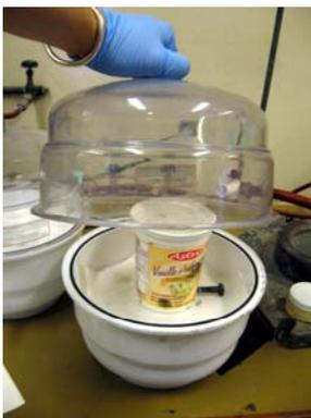
**Place the container containing the epoxy resin into the desiccator chamber and secure the lid.**
