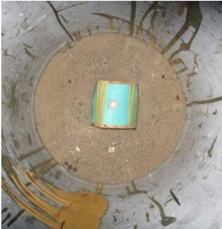
Tap the sides of the mold to make sure no air bubbles were trapped while it was pouring into the mold. You can leave your cast to cure or if you have a pressure tank, you can place the mold into the cast iron chamber, supporting the mold so it will not tip over.
