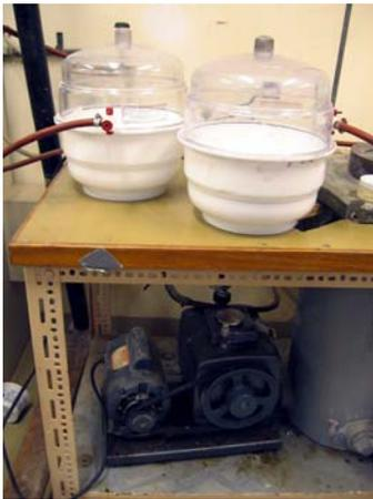
Desiccator chamber attached to a vacuum pump.
