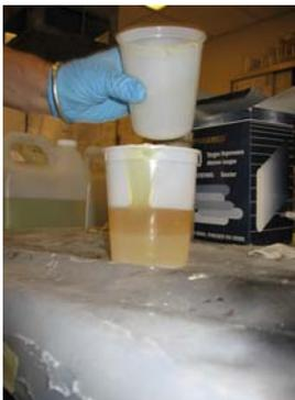
Pour Part "B" into Part "A" container. You should have a bit more epoxy resin than you need for your cast.
