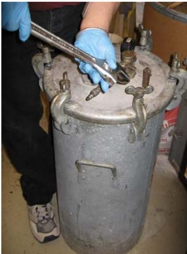
Replace the lid on the pressure tank and secure it down with the bolts.
