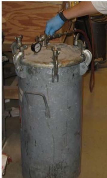
Slowly introduce compressed air into the tank until you reach your desired pressure. Any bubbles left in your epoxy resin will shrink under the increased pressure inside the tank. So if bubbles are present, they will be reduced in size and easier to patch. Once you have reached the desired pressure turn the valve off and disconnect the pressure hose and allow the epoxy to cure.
