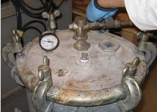
We usually increase the pressure to 40 psi. But the amount of pressure can vary depending on the type of mold used and cast made.
