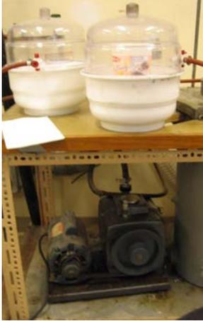
**Turn on the vacuum pump and start to evacuate the air out of the desiccator containing the epoxy resin.**
