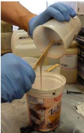
**Pour epoxy resin mixture into the container with the large screw inserted into the bottom side of the container. Make sure there is plenty of room in the container to hold up to 5 times the volume of your epoxy resin.**
