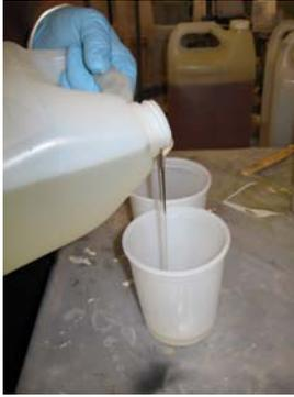
Follow the mixing instructions for your type of epoxy resin. In this example we use a 2-part epoxy resin
