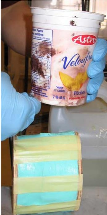
**Position your container containing the epoxy resin above the pour spout of your mold and remove the screw from the bottom of the container.**
