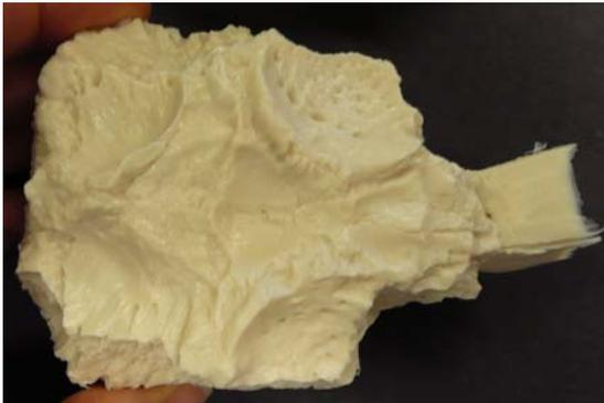
When the epoxy has cured, open your mold and take out your cast hopefully bubble free or if not, with a minimum amount of bubbles.
