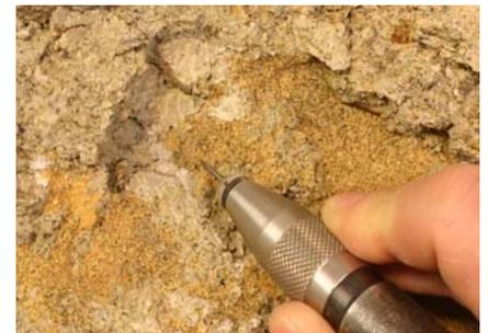
The sand was mixed with Butvar B-76 (polyvinyl butyral) in ethanol to form a cement that was pressed into the cracks and allowed to dry overnight.
